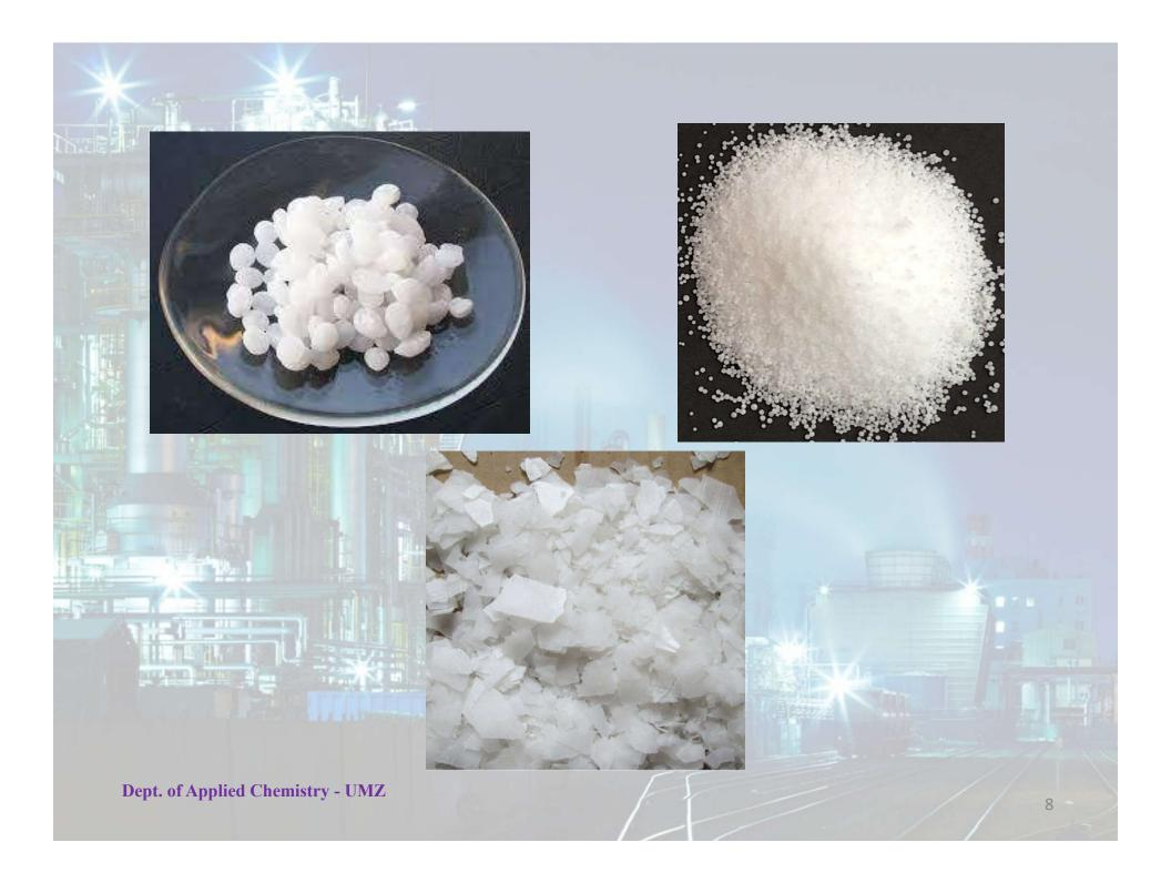
Sodium Hydroxide, or Caustic Soda, is made via the electrolysis of brine in a process known as the chlor-alkali process. During electrolysis, an electrical current is used to cause an otherwise non-spontaneous chemical reaction; in this case, the decomposition of salt.
